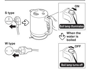
Check that the power switch is "OFF" and then unplug the plug from the power outlet.
