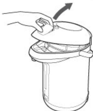
Push the front part of the **PUSH** position of the lid open lever, pick up the lid open lever, and open the lid.
