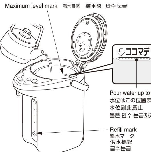
Pour in water so that the water level can stay between the Refill mark and the Max. Level mark.
