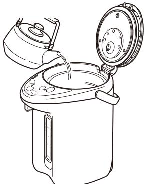
● If water of approx. 50°C or greater is poured, the automatic heating will not commence. Therefore, if this is the case, add some warm water or just water. Otherwise, you can press the Re-boil key. (For the re-boiling procedures, see page 23.)
