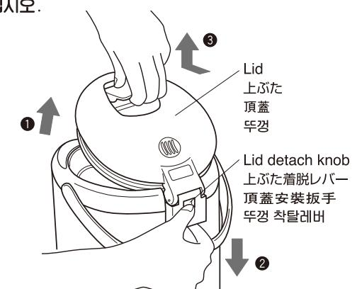
To mount the lid, press in the hook of the lid while pressing the lid detach knob.
