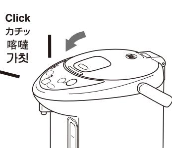
If the lid is not closed completely, boiling may not stop or much hot water may flows out when the thermo pot falls down, resulting in burns.
