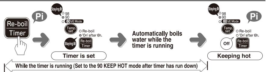
Automatically boils water while the timer is running
