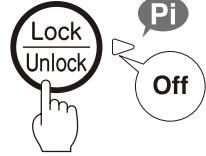
The "Unlock" lamp will switch off with a short beep, and the "Push" key will be locked. Hot water cannot be poured even if you press the key.
