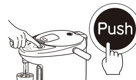
While you are pressing the key, you will hear an operation sound, and hot water will be poured through the spout. Be sure to confirm that the flow of hot water has stopped before moving your cup away from the spout.
